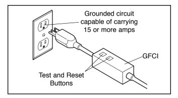
The power cord is equipped with a Ground Fault Circuit Interrupter (GFCI), located at the end of the power cord. You should always test the GFCI before using the RESTORATION 2.0.
